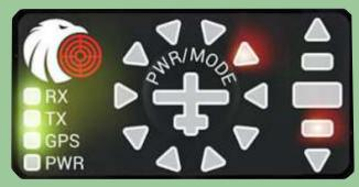
All aircraft have LED+ displays which include distance to target indication, configured at the MGC as nm (nautical miles), whereas the systems in JGE, CCZ and the Falke are more basic FLARM units and have simpler displays without distance.
