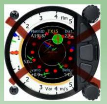
In general, FLARM units will come on when the main avionics switch is ON. In the K23 there is a separate FLARM ON-OFF switch, and the MYN FLARM comes on when the S80 is turned on. Although it is difficult to see, the FLARM (PowerMouse) in the new K21b (MYN) is connected to the S80 electronic vario, which adds more, and different, functionality.
